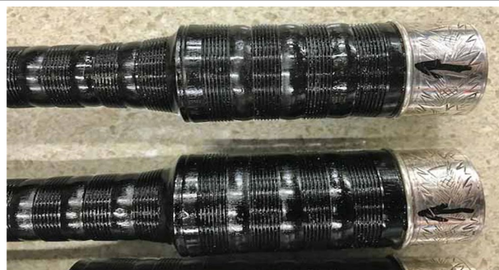
Repair completed with finish applied to the timber sections. Arrow on ferrule indicated the position of the original crack.
