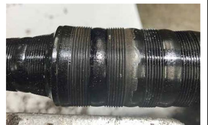
Bead area machined to match the original profile.
