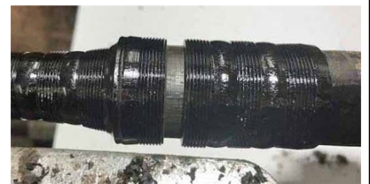
Crack filled with powdered Blackwood and specialist glue. Groove cut into raised bead area ready for whipping.
